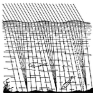
FIG. 50. Rays of sunlight penetrate the water and by the refraction of the waves are collected into lines of light. The blue rays (dotted) are more strongly refracted.
